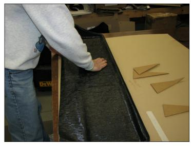
8. Pull the material towards the rear of the visor and press into place. Be sure the fit is smooth and snug.
