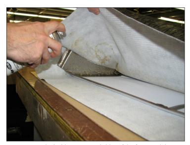
5. Now spray the inside corners and sides of the frame and the corresponding material. Let dry until "tacky".
