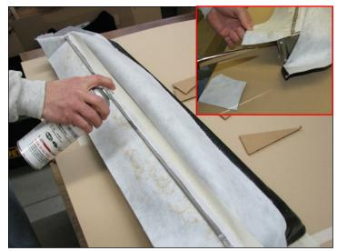
9. Turn visor right side up and spray 3/4" of the top rear edge of the frame and corresponding material, press material into place on top edge and trim. Cut the cover as shown in inset photo.
