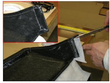
11. Trim material as shown, spray with adhesive and let dry to "tacky". Tuck around to the inside of the frame.
