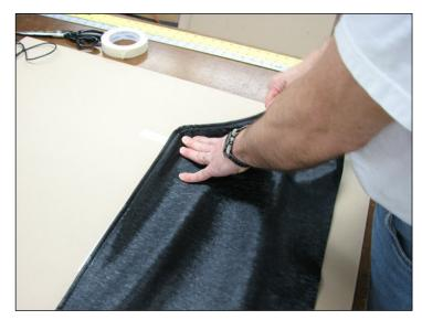
2. With the visor cover upside down slip the visor frame into the cover. Use the corners and sides to position the cover on the frame.
