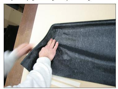
6. Line up binding with the bottom edge of the frame. Pull material towards the rear of the frame and press into place. Be sure to get the cover attached into the corner smoothly.
