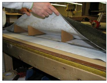
7. Lift open the cover and spray adhesive on the underside of the frame and thin cloth along with the corresponding visor material. Use triangle cardboard shims to hold the cover open while drying.
