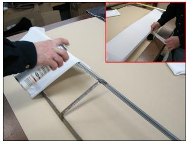
1. Attach thin cloth to the top of the visor frame using contact adhesive. Be sure to stretch the fabric tight across the center openings. Trim off excess at outside edges.
