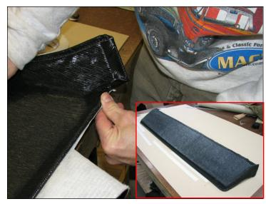
12. Trim along rear edge of visor frame and press material into place.
