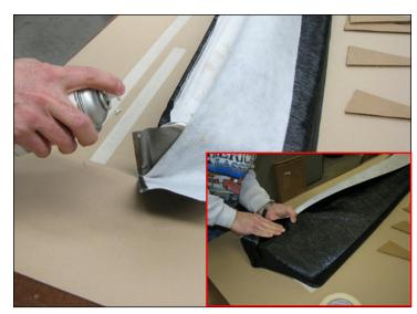
10. Next spray adhesive on outside of frame sides and material. Let dry to "tacky". Pull material up and back and press into place at sides, then work across the rear edge. Be sure that all is smooth.
